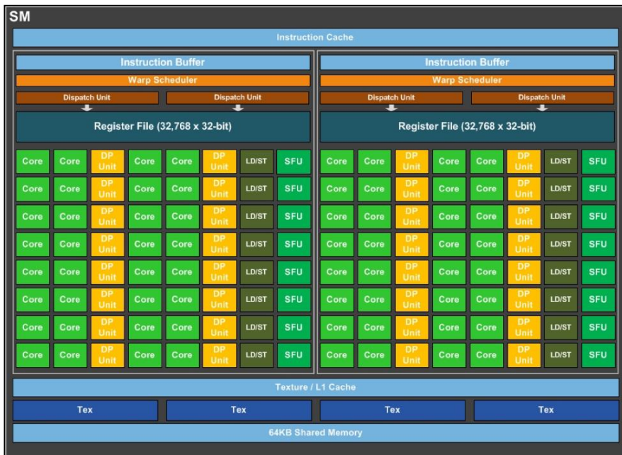
Figure 2. An overview of the latest Pascal GP100 SM architecture 1
